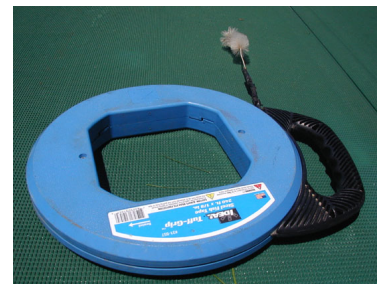
Bottle brush w/ plumber or electrician's snake
